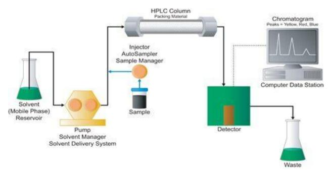
Figure 4 Schematic Diagram of HPLC chromatogram at AIGLENT TECHNOLOGY
